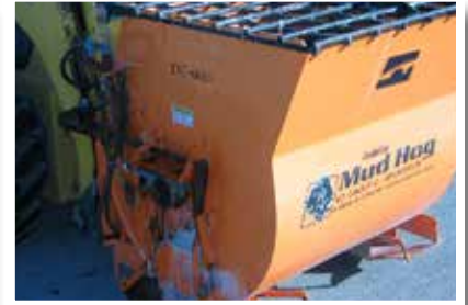
Mixing/laying equipment can be used to lay Elephant Armor
